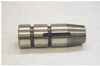
Example: Externally Strain Gauged
