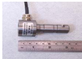
Example: Internally Strain Gauged
