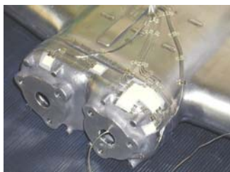
Ceramic installation with additional custom made K Type thermo couples.
