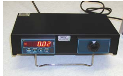
Housed in an enclosure with an 8 way memory switch
