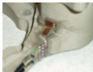
Strain Gauging Plastic—Two part epoxy adhesive
