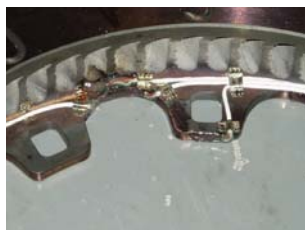
Strain Gauging Plastic—Two part epoxy adhesive
