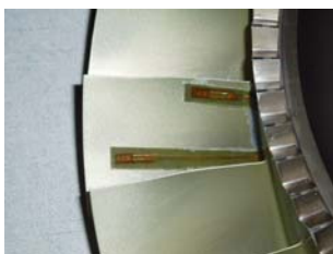
Strain Gauging Steel— Epoxy-phenolic adhesive
