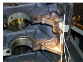
Strain Gauging Steel— Standard Installation
